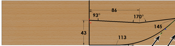
Fig. 10 Ctrl click Circular Spline Handle and edge
